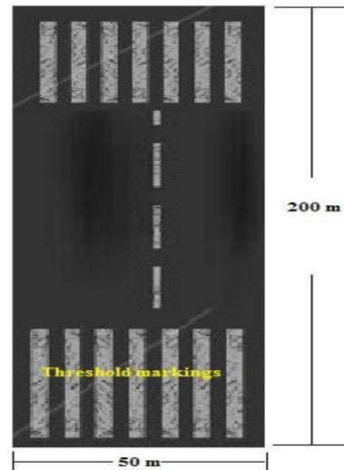
Figure 7. Threshold markings
