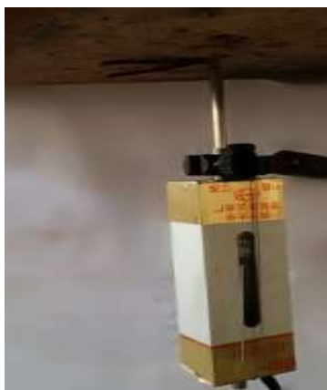
Figure 1(b).Experimental method for deflection measurement
