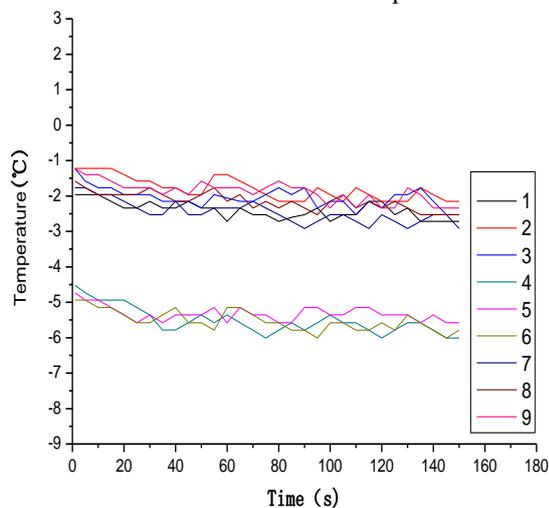
Figure 9. The temperature variation of measuring points at the central area of beam of T12
