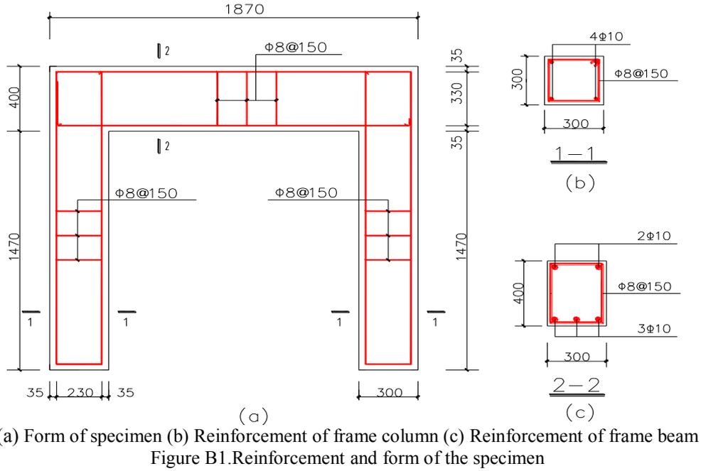
Figure B1. Reinforcement and form of the specimen
