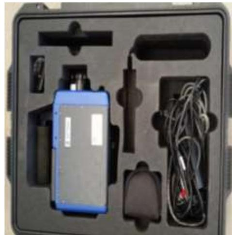
Figure 7(a). Thermal infrared imager SC7000
