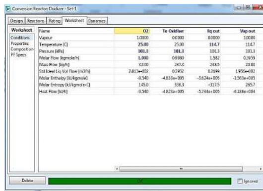
Figure 2.HYSYS result for oxidizer
