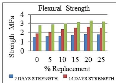
Figure 7.Comparison of flexural strengths
