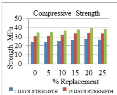
Figure 5.Comparisons of compressive strengths
