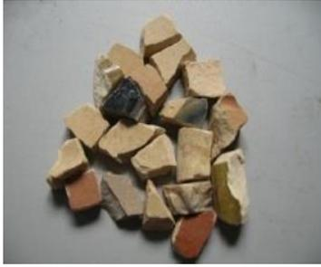
Figure 1. Ceramic coarse aggregate
