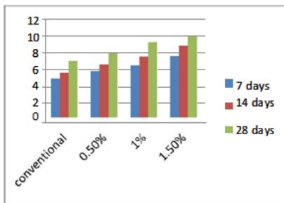
Figure 3. Comparison of flexural strength of concrete
