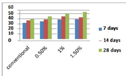
Figure 1.Comparison of compressive strengths of concrete
