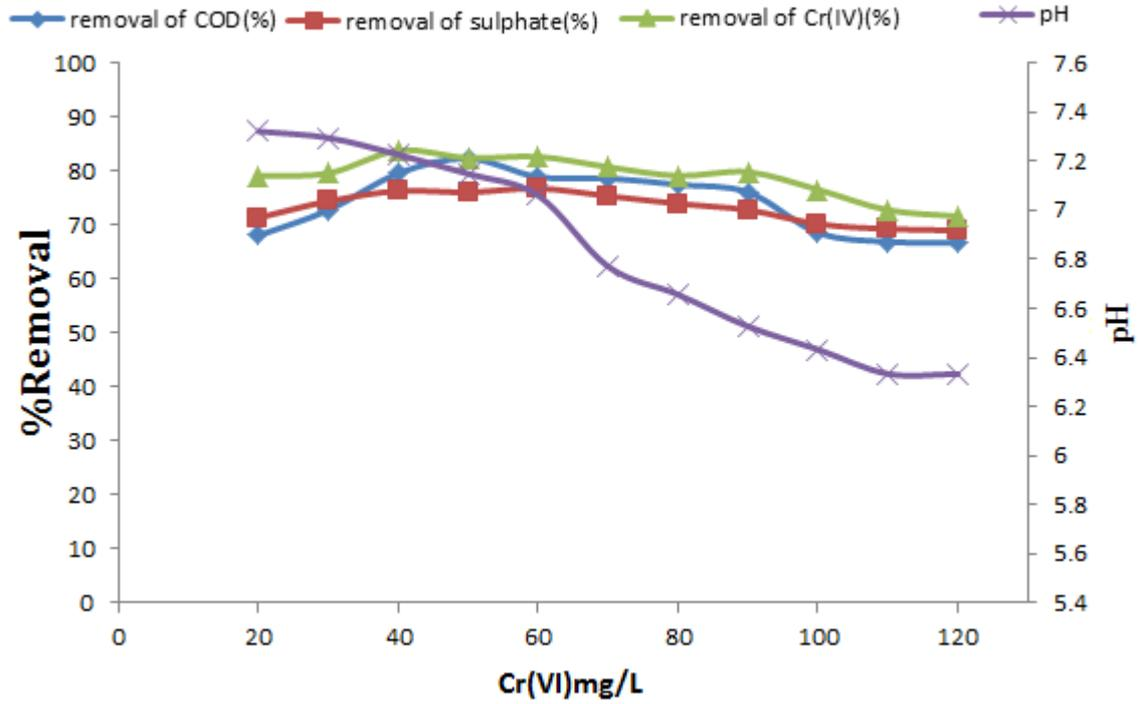
Figure A3.Initial metal dose consequence on various parameters reduction at pH 7 in optimized and temperature 37 ° C and time 7 days of incubation.
