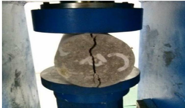
Figure A2. Testing of split tensile strength
