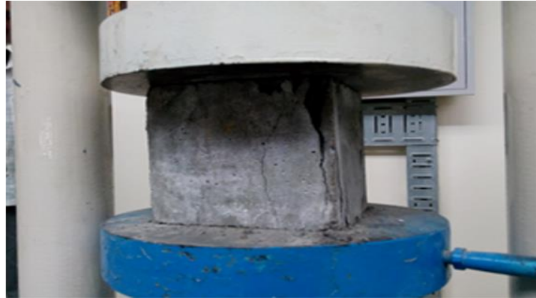
Figure A1. Testing of compression strength
