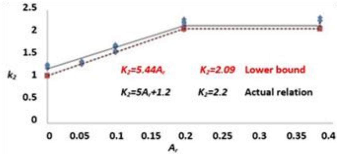
Figure B1. Variation of FSAF ( $k_2$ ) with area ratio ( $A_r$ ) at collapse for all RCC-GFRP composite beams
