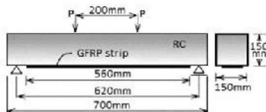
Figure 1. Details of the RCC-GFRP composite beam test specimens.
