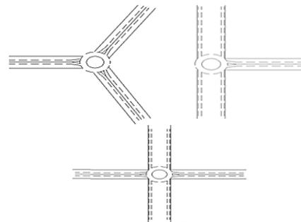
Figure 1. Rough alignment for 3 and 4 road junctions
