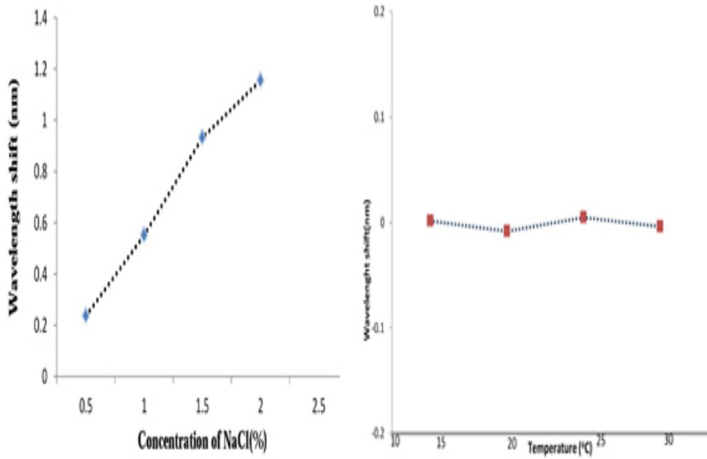
Figure A3.LPG Wavelength shift due to variations in concentration of NaCl at 30 °C (left) and temperature compensated Wavelength shift of the LPG due to temperature varying at 1 % concentration of NaCl (right).
