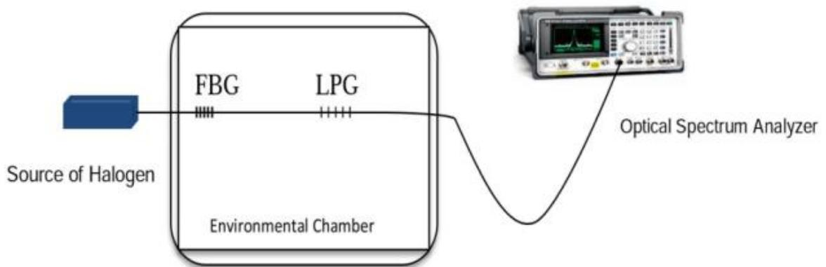
Figure A1. Experimental setup for calibration of temperature
