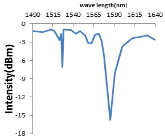
Figure 1.FBG/LPG hybrid sensor transmission spectra
