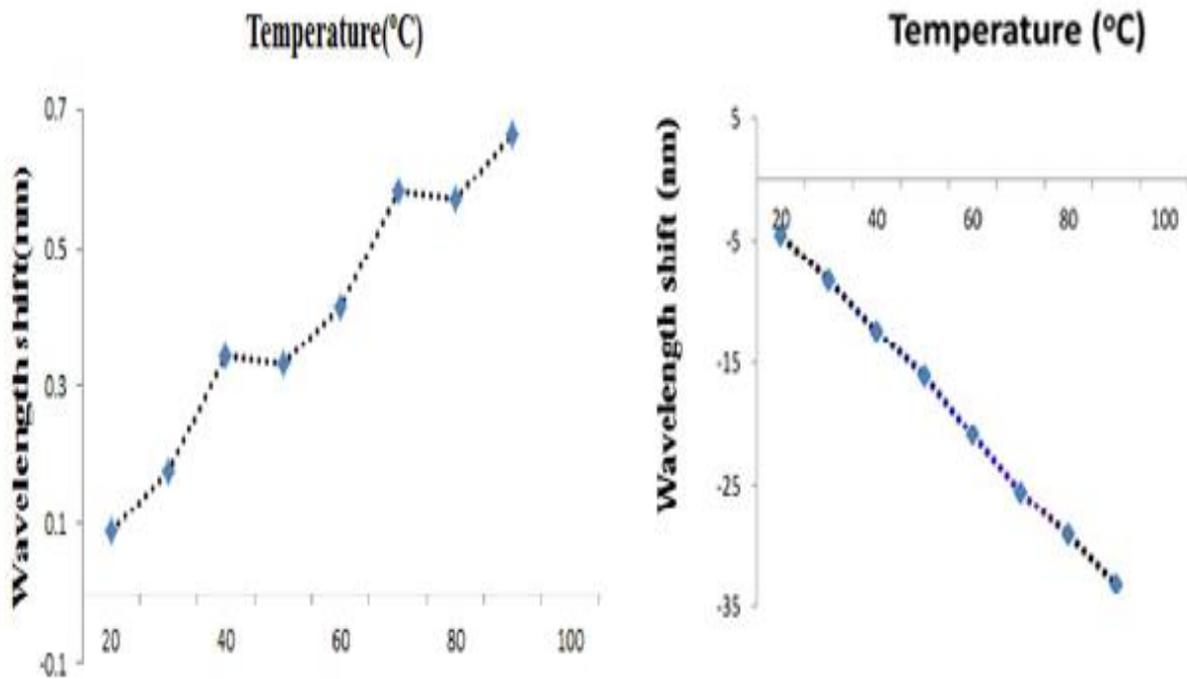
Figure A2. Variation of temperature on the bare hybrid sensor, Performance of FBG (left) and LPG (right)
